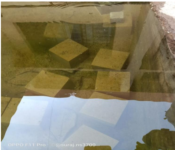
Fig No-6 Curing of Specimens
