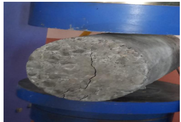
Fig No-7 Testing of Specimen
