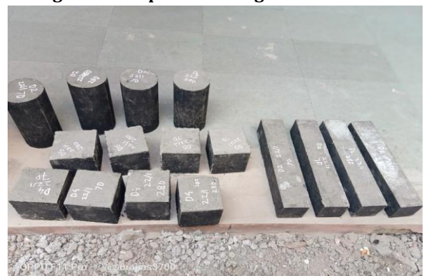
Fig No-5 Cubes, Beams and Cylinders
