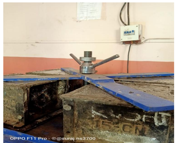
Fig No-4 Compaction Using Table Vibrator
