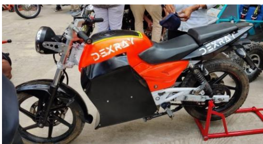
Fig -7: The retrofitted bike for with Li-ion battery
