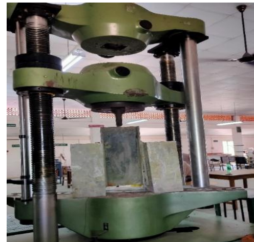
Fig -5 Test setup for Monotonic loading
