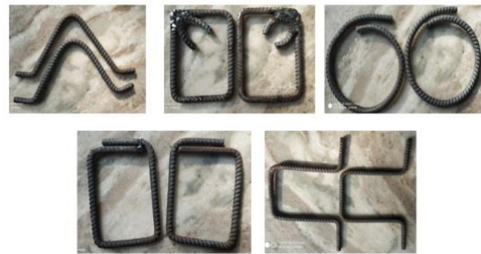
Fig -1 Rebar shear connectors; (V shape, Closed stirrups, Circular spiral, Rectangular spiral, and Open link respectively)
