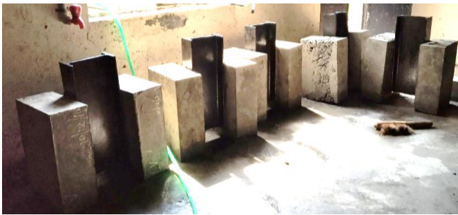
Fig -4 Specimen cast for Monotonic loading
