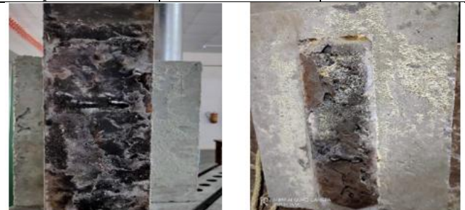
Fig -6 Failure type in specimen: connector part attached to (a) steel beam (b) concrete
