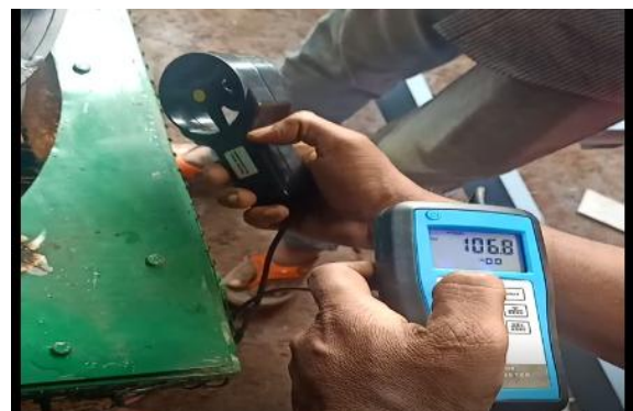
Fig-17 Testing using wind anemometer
