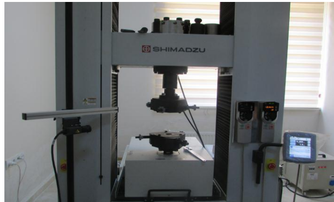
Fig. 4: Test setup for the torsion test
