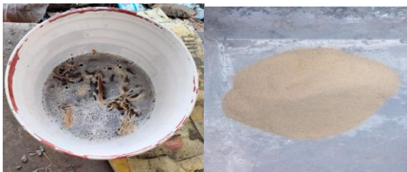
Fig.3.3: Alkali Treatment of Fibres
