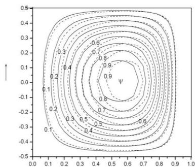
**Fig.4.** Comparison of the cell pattern at the onset of instability for  $\beta = 1.0$  (shown by continuous curve) and  $\beta = -1.0$  (shown by broken curve) at constant  $N = -0.4$ .
