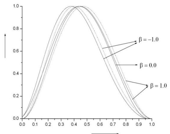
**Fig.6.** The radial eigenfunction  $u(x)$  for  $N = -0.2$  (shown by broken curve) and for  $N = -0.1$  (shown by continuous curve) for different values of  $\beta$ .
