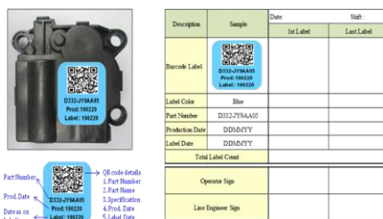
Figure 16. Barcode attached to the part
