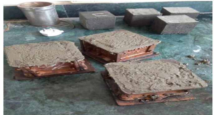
Fig -1: Casting of Cube
