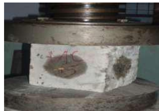
Fig -3: Compressive Strength Testing Arrangement
