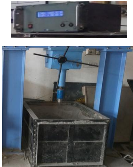
Fig. 5 Model tank Experimental set up for Load - settlement and load cell indicator
