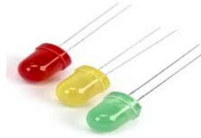
Fig.5: LED's used for traffic control
