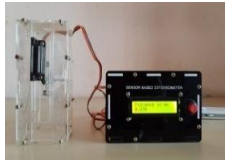
Fig.4-Developed Sensor Based Magnetic Extensometer
