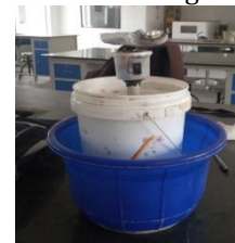
Fig -8: TRICKLING FILTER MODEL
