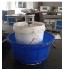
Fig -10: TRICKLING FILTER MODEL
