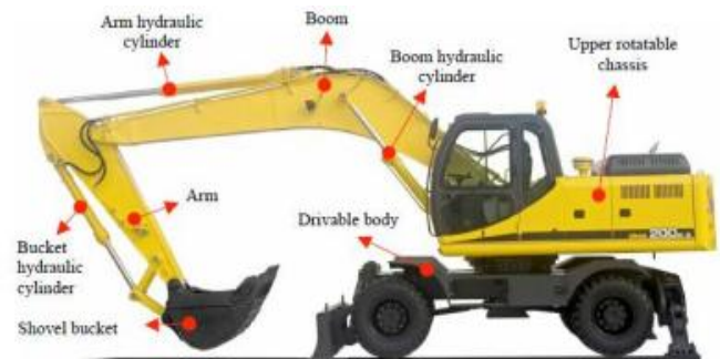
Fig.1: General view of an excavator
