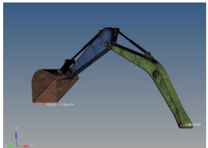
Fig.20: Meshed model of assembly for iteration IV
