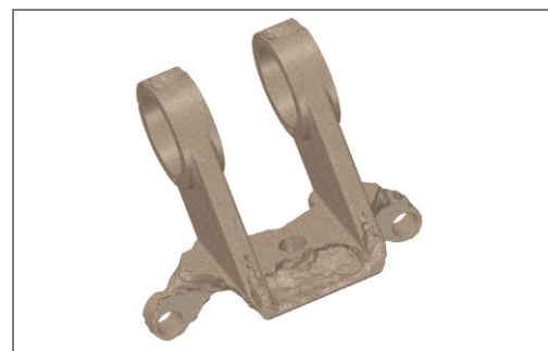
Fig. 8 Optimized design at 46.65 % mass reduction
