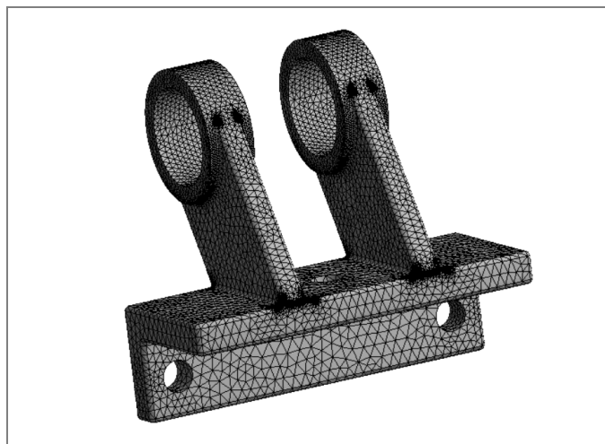
Fig. 3 Meshed model of the bracket
