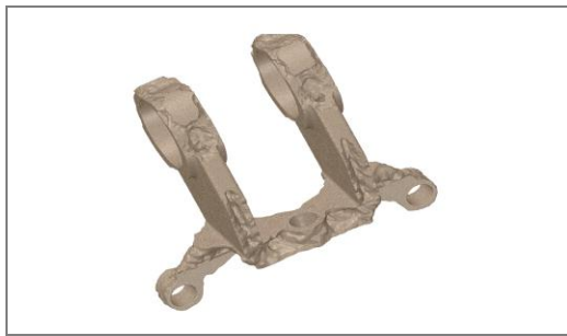
Fig. 10 Optimized design at 65.5 % mass reduction
