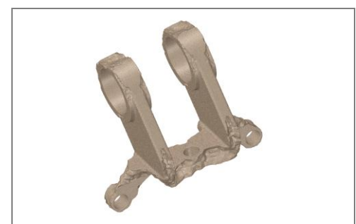
Fig. 9 Optimized design at 55.84 % mass reduction
