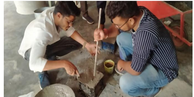
Fig -4: Casting by Steel Moulds
