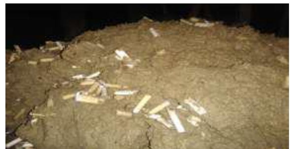
Fig-1 MIXING OF CB's AND CLAY
