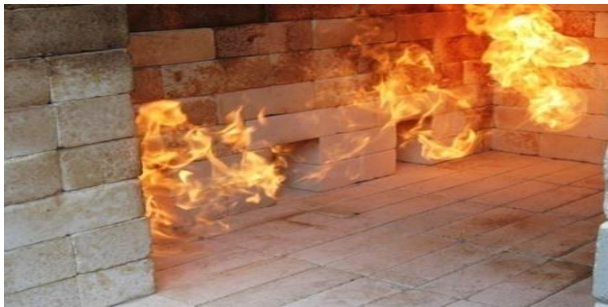
Fig-5 Bricks in kiln
