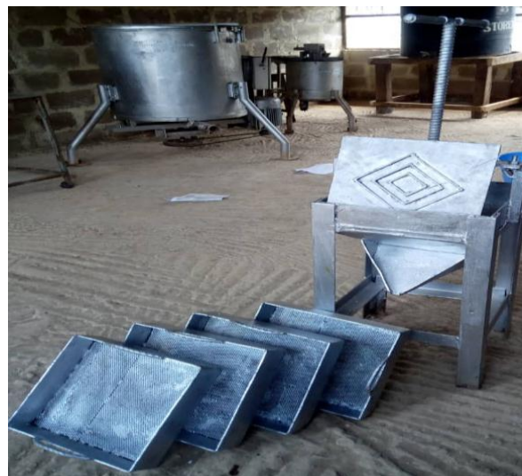
Plate 3: Wall panel moulding machine
