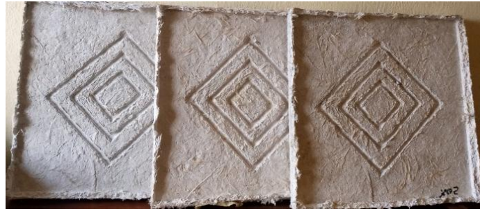
Plate 4: Moulded wall panels before trimming
