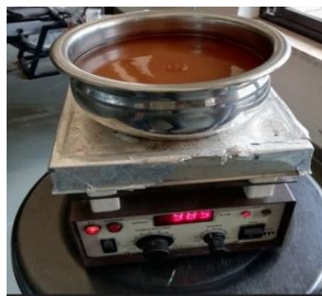
Fig -6: Mixing of lye and oil using magnetic stirrer
