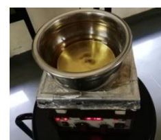
Fig -12: Drying of biodiesel
