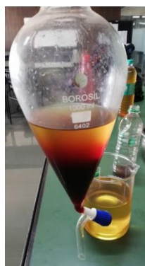
Fig -9: Separation glycerol and biodiesel using separation funnel
