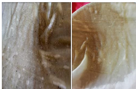
Fig -3: Trapped contaminant
