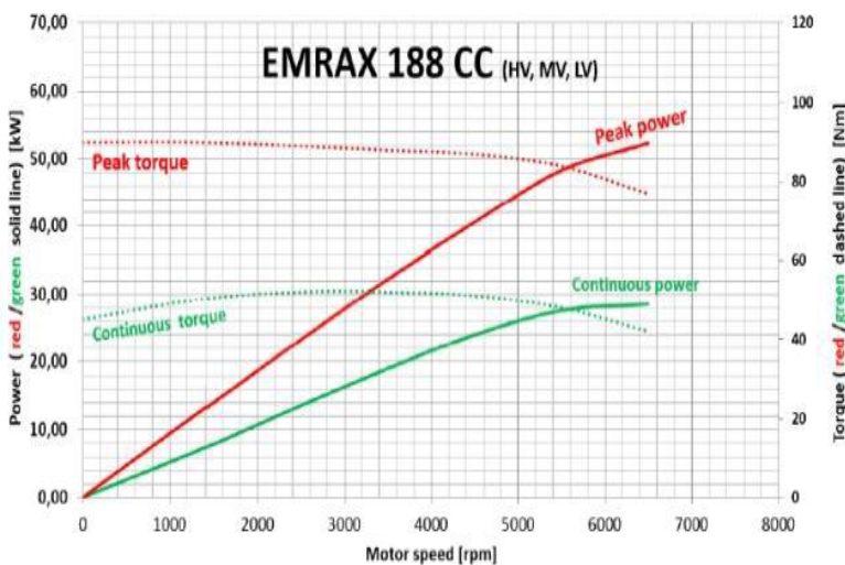
Chart -1: Plot of power V/s torque V/s motor speed for an EMRAX motor
