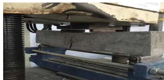
FIG. 5: Failure crack appearance in the flexural strength test
