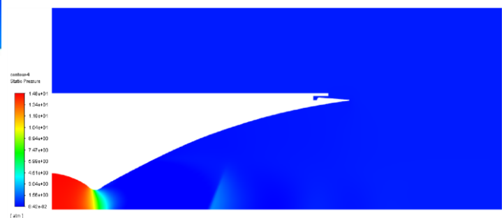
Fig-16: 15 atm main nozzle pressure inlet static pressure
