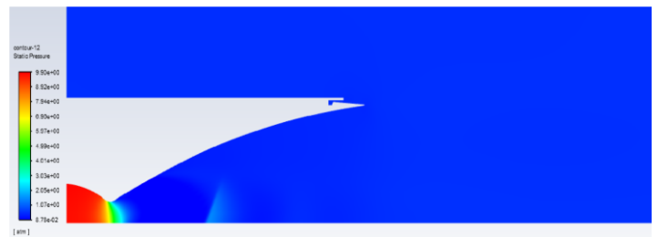
Fig-13: 10 atm main nozzle pressure inlet static pressure
