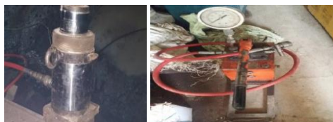
Fig 3.3 hydraulic jack and pump
