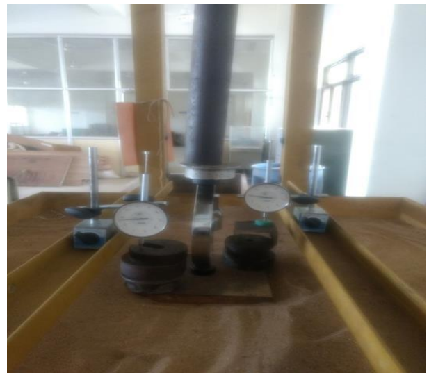
Fig- 8: Plastic cups beneath the test plate arrangement
