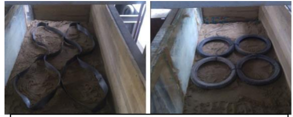
Fig- 1: Geocell and Waste tires
