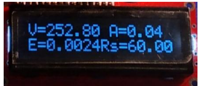
Fig -3: Current consumption information is displayed on LCD
