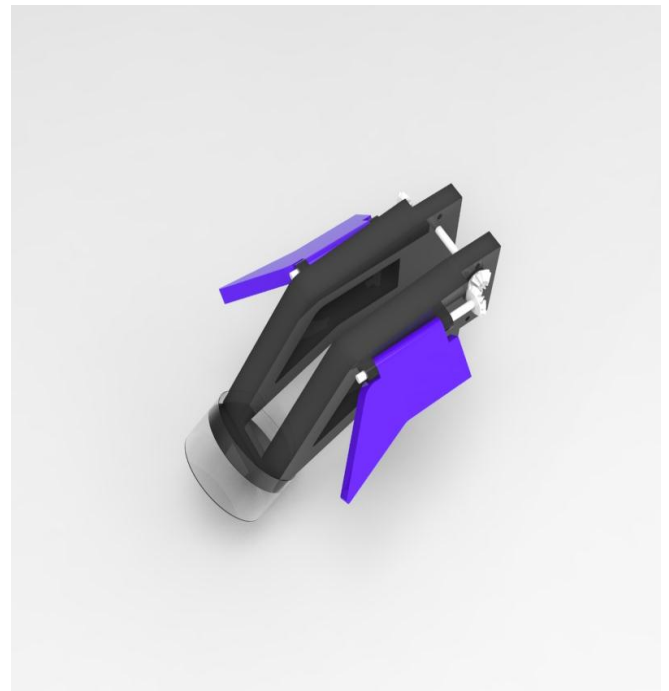
Fig -13: Isometric view of the final leg design with flaps and piezo electric sensor.
