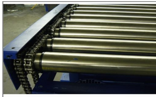
Fig. Roller conveyor (Chain Type)
