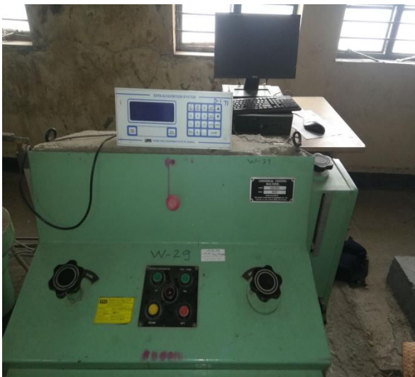
Fig4.2 Load control Unit
