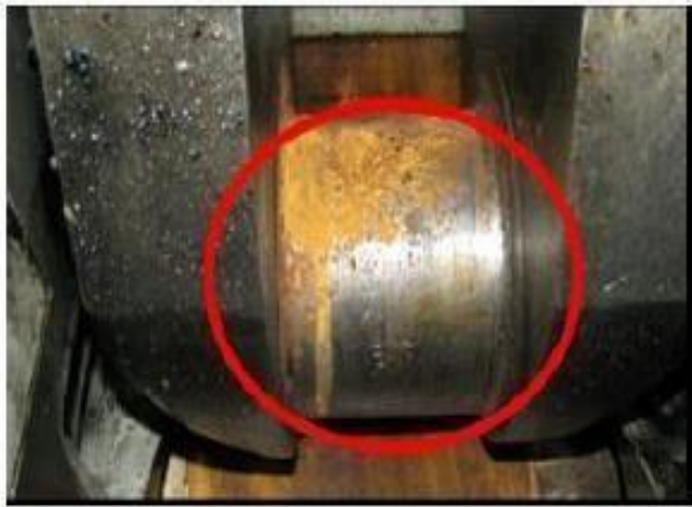
Fig -2: Failure in surface hardening [12].
