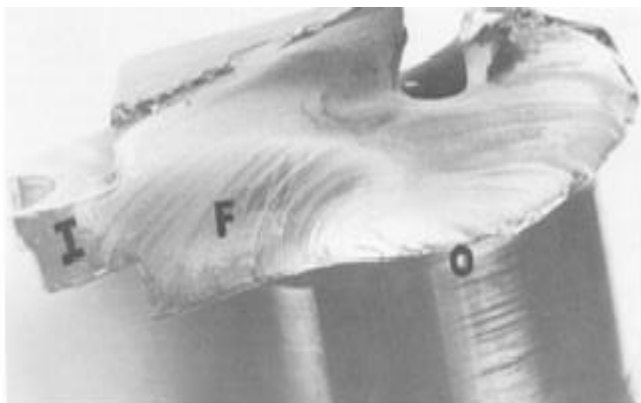
Fig -3: Failure in Bending.
