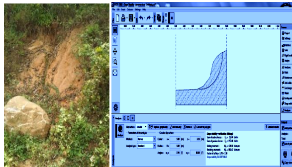
Fig -2: Analysis of slope 1 from FEM based software GEO 5
