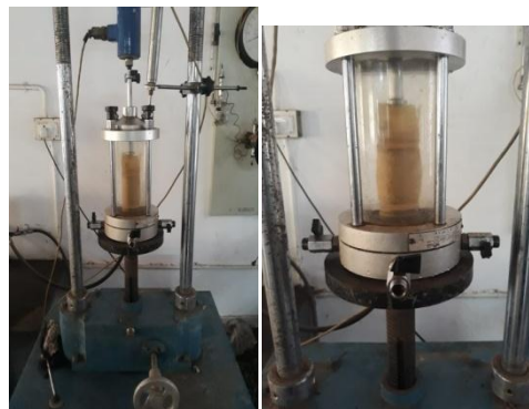
Fig.1 Triaxial testing on sample before & after Loading
