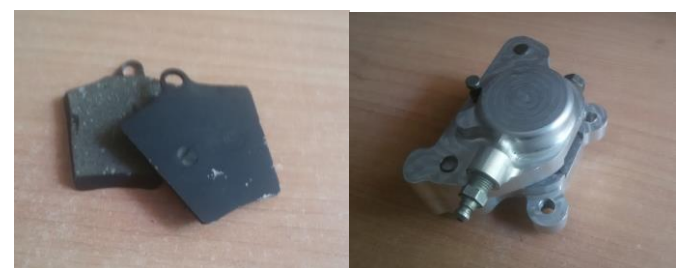
Fig -13: final product brake pad & brake caliper
