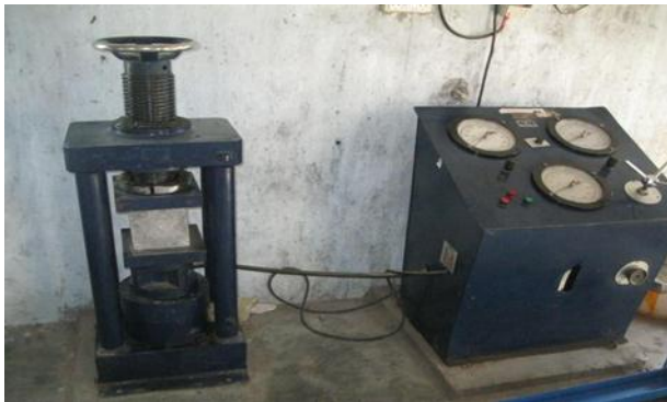
Figure 4.2: Compressive Strength Testing Machine (2000KN)
