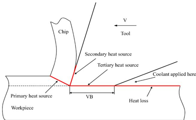
**Fig.1.1** Sources of heat generation in orthogonal cutting process.
