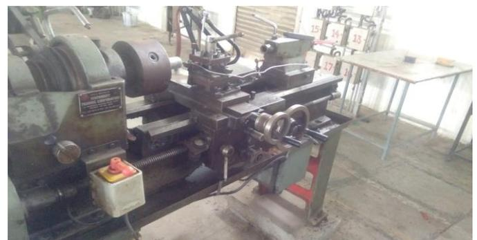
**Fig.2.1** Centre lathe machine
