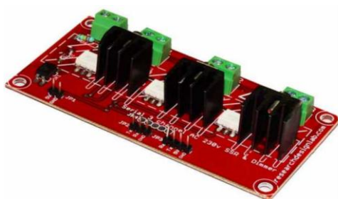
Fig 7: 3 Channel AC Dimmer
