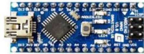
Fig.4. Arduino Nano Board
