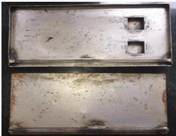
Figure -2: Metal template for casting(400*200*15 mm)
