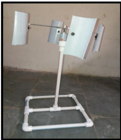
Fig -1: Prototyped Vertical Axis Wind Turbine.
