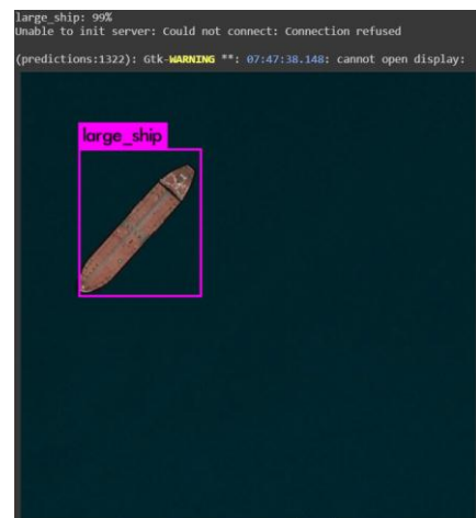
Confidence: 99% Total Execution Time: 40.67ms Computation Resources used: 65.33 BFLOPS
