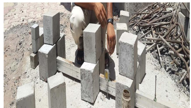
Figure: 8 Measurement of Pavement Curling with Extensometer
