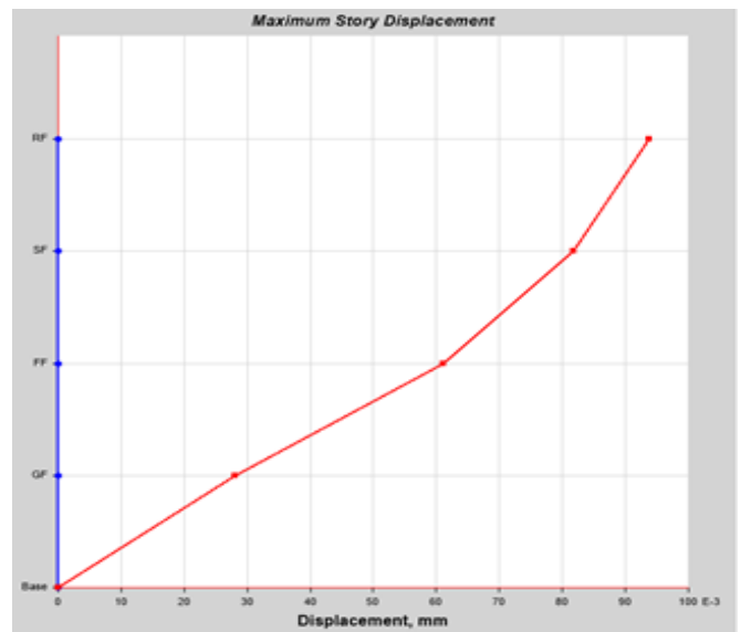
Fig -1: Story Response- Maximum Story Displacement for RCC Model
