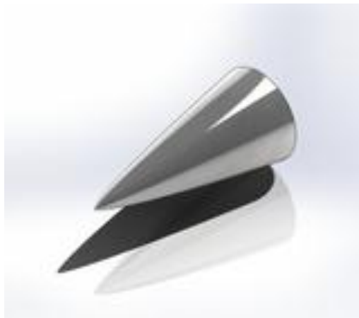
Fig-2 power series nose cone, n=3/4 .
