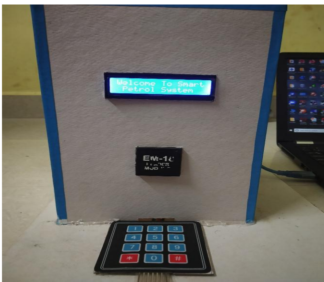
Fig: 5.1.1 Display part along with RFID scanner and keypad
