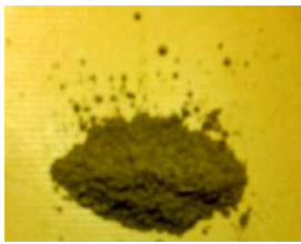
Fig - 2 : Shows dust collected on PV panels
