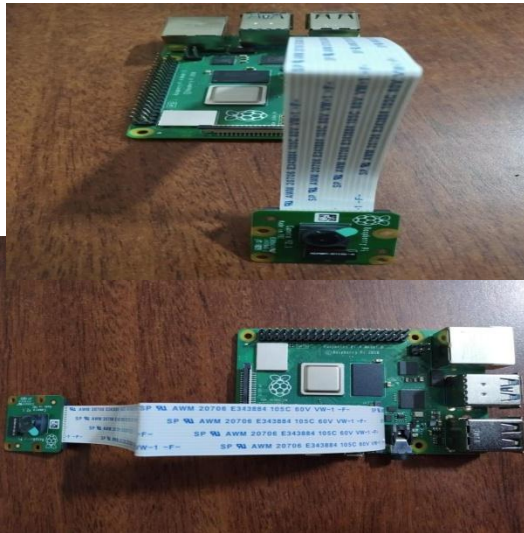
Fig17: Raspberry Pi 4b model connected to Raspberry Pi Noir camera
