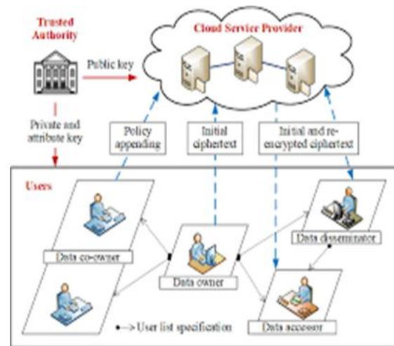
Fig -1: System model of proposed scheme. The user role is divided into the following categories: data owner, data co-owner, data disseminator and data accessor
