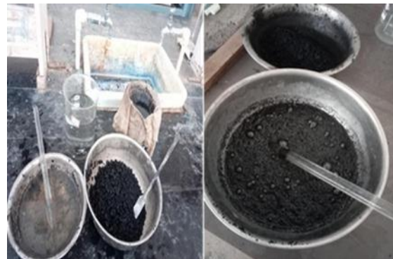
Fig. 3: Blast furnace burnt groundnut shell powder with sulphuric acid
