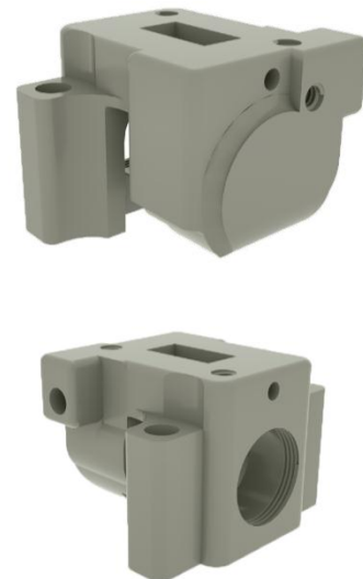
Fig -4: Final design of brake caliper body
