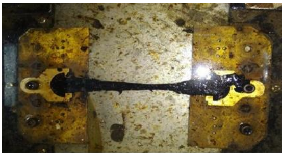
Fig -1: Ductility Test of Modified Bitumen
