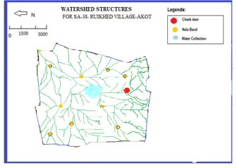
Fig -2 Water Harvesting Structures for Ruikhed Watershed
