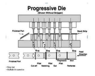
Progressive stamping may be a metalworking method which will encompass punching, coining, bending and a number of other ways of modifying metal staple, combined with an automatic feeding system.
