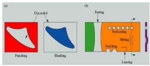
Fig.1.Shearing Operations: Punching, Blanking and perforating
