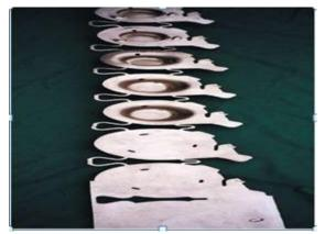
Figure 8: The parts shown here are carried by the scrap between them, which also serves as stretch webs for the center draw.
