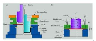
Fig.4. Schematic of the Drawing process.
