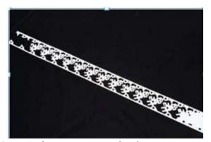
Figure 6: This part was rotated in the strip to maintain critical tolerances better .
